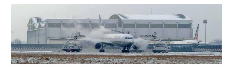
In winter, the ice that builds up on an aircraft fuselage and wings will make it too heavy and therefore much harder to fly; this could in turn have serious consequences when taking off. For obvious safety reasons, the aircraft's captain may decide to request the de-icing of the aircraft.
